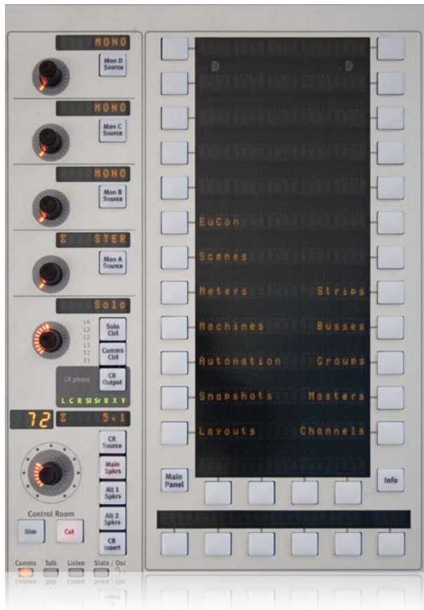
Monitor Section and the Main panel to the right. Main panel shows the Main Menu with all the major section headings
